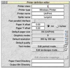
Figure 1: The UniPrint driver as supplied, loaded into PrintEdit
