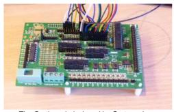
The Gertboard, designed by Gert van Loo, provides an easy way to interface with a Pi
