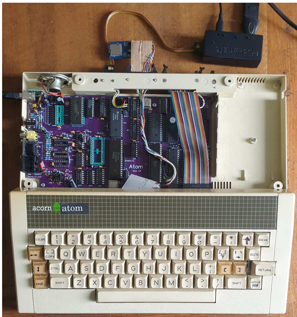
The populated replica Atom board installed in the Electron case, with the expanded keyboard
